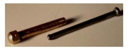
2. Cut off threaded part of bolt allowing 4" long.
