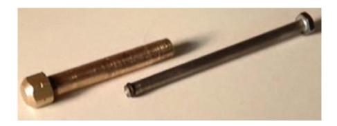
7. Fire Piston is ready to use. Put some cloth or burt cloth into the end of the bolt and insert into barrel and compress fast and hard.
