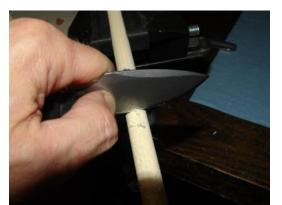
A knife can be used as a scraper to remove material quickly from the dowel.
