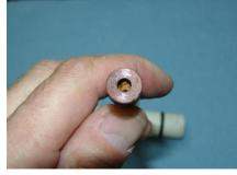
Now drill a hole into the end of the plunger. Using a 1/4" bit and going about 3/8" deep is a good starting point. Since this design gives some much volume and compression, the hole isn't all that critical.
