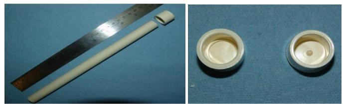
While boring an acceptable hole in a piece of wood or plastic isn't always easy, making the cylinder from CPVC is a trivial exercise.
