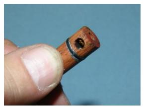
Here are some ideas for non-traditional holes. A hole that goes across the dowel makes for easier removal of the tinder. This particular plunger has a hole in both dimensions. The thought here was that the hole in the end would better expose the tinder to the high pressure/temperature air, and the hole in the side would make it easy to pop out the tinder. This worked out well.
