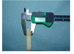
Step one is to check whether the dowel fits inside of the 1/2" CPVC pipe.
