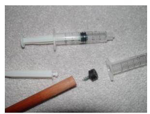
But... the syringe does have one redeeming quality, the rubber seal is perfect! Pull the plunger out of the syringe and remove the rubber seal.
