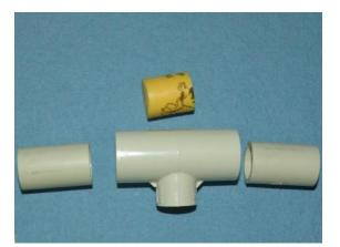
The first construction step is to cut the cork in half and press-fit it into the 3/4"-1/2"-3/4" T Fitting.
