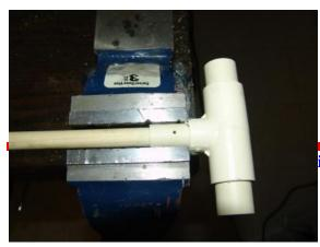
Now we cut the dowel to size, and insert it into the T handle. The length of the dowel should be such that it "just" touches the bottom of the cylinder. Any air-space left over is a bad thing
