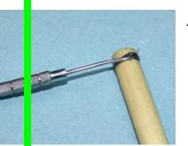
A dental pick is a useful tool for removing the O-ring from the slot.
