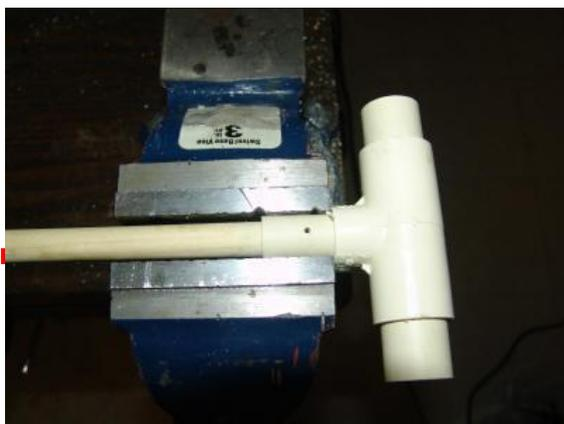
Now we cut the dowel to size, and insert it into the T handle. The length of the dowel should be such that it "just" touches the bottom of the cylinder. Any air-space left over is a bad thing
