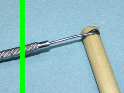
A dental pick is a useful tool for removing the O-ring from the slot.
