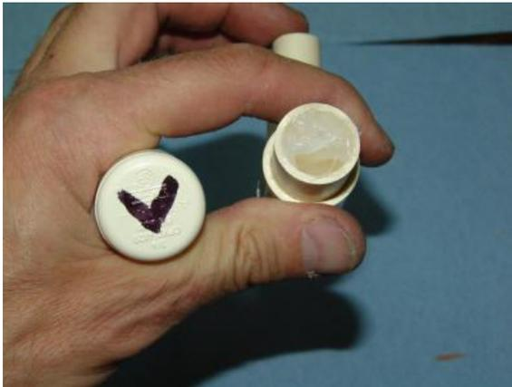
Removing the other end-cap show where Vaseline is stored. The Vaseline is used to lubricate the plunger O-ring. It can also be applied to cotton balls or other organic material and makes a great fire-starter.
