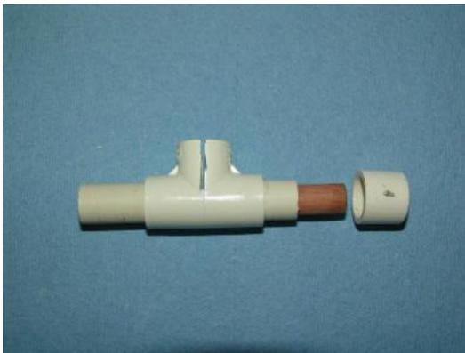
Here is a partially assembled version of the jig. Note the slot that has been sawn into the T-fitting.
