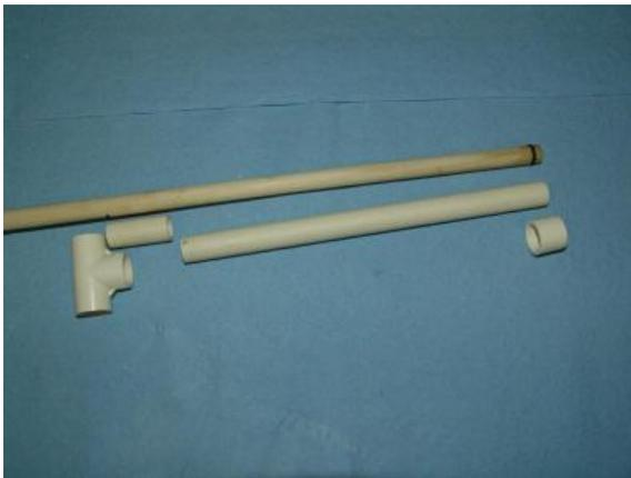
This is the trickiest part of the whole project - the plunger itself. We are going to use an O-ring to provide an air-tight seal to the cylinder.
