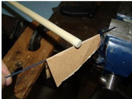
When dowel with O-ring can be forced in the cylinder, it's time to smooth out the slot with some sandpaper. One technique to do is fold some sandpaper over a piece of string. It is important not to remove too much material during the sanding process.
