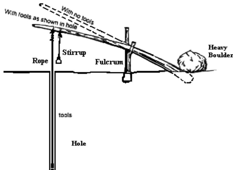
The principle which the spring pole employs is reciprocation. The down-stroke is accomplished by leg power using the stirrup. The pole then springs back (reciprocates) to its normal position which depends on the weight of the drill string and wood or metal rod.
